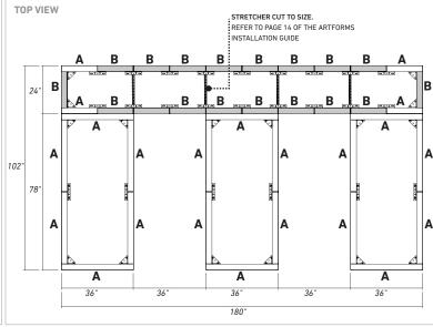
**REQUIRED HARDWARE** JOINING PLATE 48x OUTER CORNER 32x INNER CORNER 0x 2x
