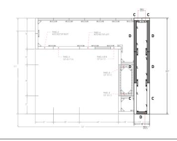
**REQUIRED PANELS** 18 x 36 PANEL 10x 18 x 36 PANEL 23x 5x IMPORTANT: 18 x 36 panels are sold in pair/layer or in full pallet only. 6 x 36 panels are sold per unit or in layer or in full pallet. **REQUIRED HARDWARE** ANCHOR SLIDE AND NUT 150x JOINING PLATE 22x OUTER CORNER 6 x
