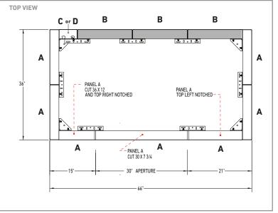
**REQUIRED HARDWARE** ANCHOR SLIDE 40x AND NUT JOINING PLATE 8x OUTER CORNER 0x INNER CORNER 0xSTRETCHER
