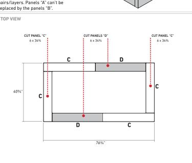
0x**6**x **4**x 2xIMPORTANT: 18 x 36 panels are sold in pair/layer or in full pallet only. 6 x 36 panels are sold per unit or in layer or in full pallet. **REQUIRED HARDWARE** ANCHOR SLIDE 56x JOINING PLATE 14x
