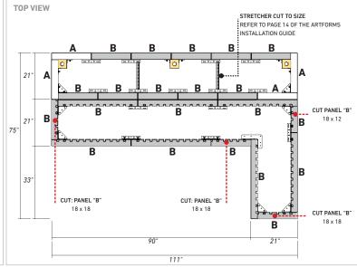
0x0x IMPORTANT: 18 x 36 panels are sold in pair/layer or in full pallet only. 6 x 36 panels are sold per unit or in layer or in full pallet. **REQUIRED HARDWARE** ANCHOR SLIDE 116x JOINING PLATE 40x OUTER CORNER 14x INNER CORNER 2x1x
